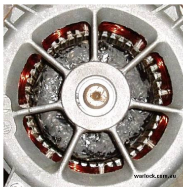
Figure 5. Completed conversion a 1/4 hp induction motor
