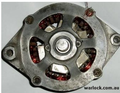
Figure 4. Completed conversion of the 40 Amp car alternator
