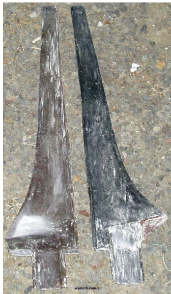
Figure 9. Negative moulds of wind turbine blades
