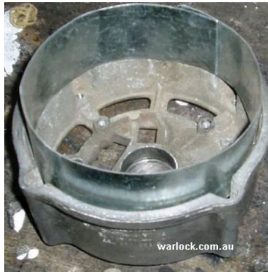
Figure 3. 40 Amp car alternator stator with shielding
