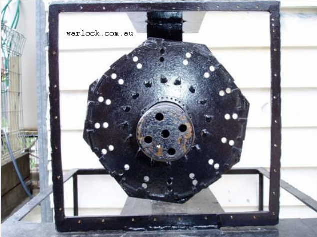
Figure 1. Rear half of the generator motor
