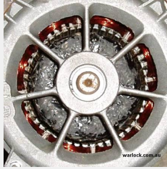
Figure 5. Completed conversion of a 1/4 hp induction motor
