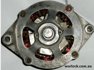
Figure 4. Completed conversion of the 40 Amp car alternator
