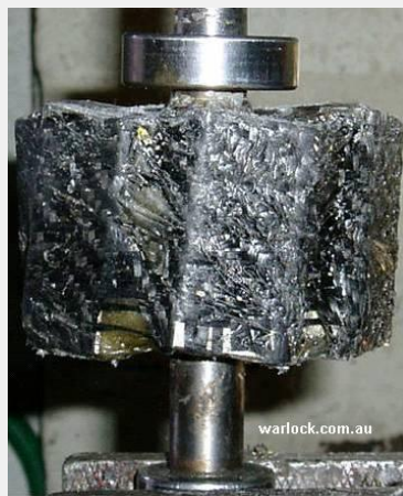
Figure 2. 40 Amp car alternator rotor with magnets fibre glassed in place
